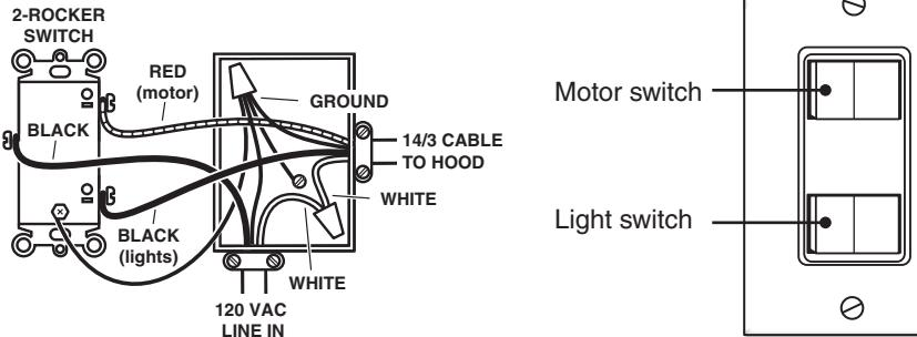
**NOTE:** Allow enough length of 14/3 cable to perform the RED wire connection in the hood nose.
