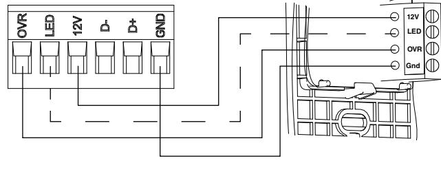
NOTE: The auxiliary wall control can be used with a 3-wire connection by removing the LED signals. This optional wiring will not allow an installation with more than 1 auxiliary wall control to properly synchronize their LEDs on an event requested from a peer. Only the auxiliary wall control having requested the timer event will have the LEDs updated accordingly.
