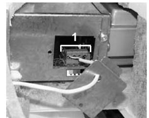
**NOTE:** Push forward slightly on the little tabs (1) to ease insertion of each wires.
