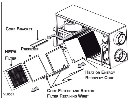
\*Bottom filter retaining wire only on H50100E unit.
