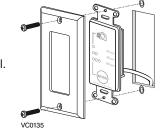
Perform the electrical connection to the terminal connector of the unit, as shown below. For more details, refer to the installation manual of the ventilation unit.
