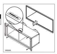
Assemble the grille to the metal tandem hood box using both  $n^{\circ}$ . 8 x 3/8" screws previously removed plus 2 other  $n^{\circ}$ . 8 x 3/8" screws from parts bag. Seal the outline with caulking.
