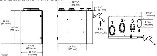
NOTE: ALL UNITS PORTS WERE CREATED TO BE CONNECTED TO DUCTS HAVING A MINIMUM OF 6" DIAMETER, BUT IF NEED BE, THEY CAN BE CONNECTED TO BIGGER SIZED DUCTS BY USING AN APPROPRIATE TRANSITION (E.G.: 6" DIAMETER TO 7" DIAMETER TRANSITION).
