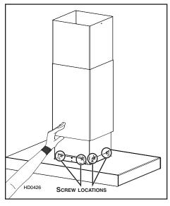
Slide the lower flue down on top of the hood and secure from inside the hood using 4 no. 8 x 3/8" quadrex screws (included).
