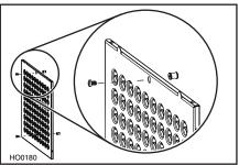
Rest rear filters edge on filter springs in the range hood. Using knob, tilt up the filters into position. Make sure filter tabs are securely engaged in range hood front edge after installation.
