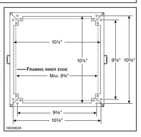
Finish ceiling surface. Be sure to mark the location of the ceiling joists and cross framing. Bring house wiring through finished ceiling.
