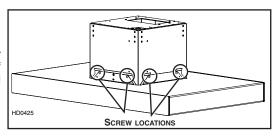
Lift flap located on top right hand corner of blower box (1) to ease wire clamp installation (included). Install wire clamp and push flap back in place. Secure flap to blower box (2) using 1 no. 8 x 3/8" quadrex screw.
