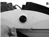
2 Splice back the end of the cable to access the 4 wires. Strip the end of each wire. Insert the end of the cable through the small hole on the front of the unit.
