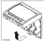
• RUN THE CABLE (4 WIRES) THROUGH THE CENTRAL OPENING OF THE MOUNTING PLATE AND MOUNT THIS PLATE TO THE WALL USING SCREWS (NOT INCLUDED). IF NEEDED, USE WALL ANCHORS (NOT INCLUDED).
