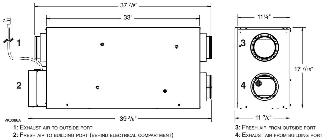
NOTE: All unit ports were created to be connected to ducts having a minimum of 5" diameter, but if need be, they can be connected to bigger sized ducts by using an appropriate transition (e.g.: 5" diameter to 6" diameter transition).
