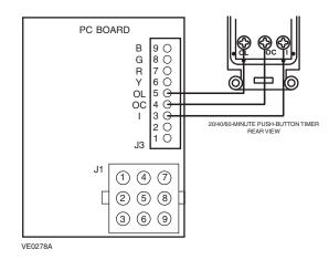
Plug the ventilation unit and test the push button.
