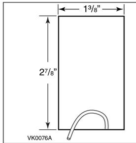
3 TEMPORARILY PLACE THE SWITCH OVER THE HOLE AND MARK BOTH MOUNTING SCREW HOLE POSITIONS.
