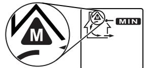
**RESETTING MAINTENANCE INDICATOR:** PRESS SIMULTANEOUSLY ON BOTH ARROW BUTTONS, MAINTENANCE INDICATOR WILL DISAPPEAR FROM LCD SCREEN.
