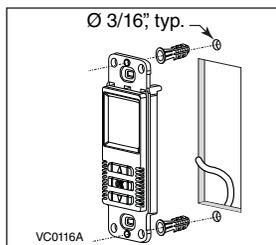
5 STRIP THE END OF THE CABLE TO ACCESS THE 4 WIRES. STRIP THE END OF EACH WIRE. USING A SMALL BLADE SCREWDRIVER, CONNECT EACH WIRE TO ITS CORRESPONDING TERMINAL, ON THE BACK OF THE WALL CONTROL: YELLOW WIRE TO "Y"; RED WIRE TO "R"; GREEN WIRE TO "G" AND BLACK WIRE TO "B".
