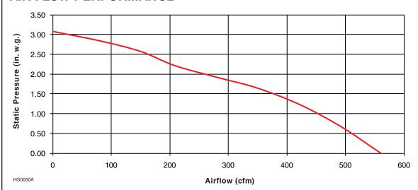
® 2100 L HVI CERTIFIED HVI-2100 CERTIFIED RATINGS comply with new testing technologies and procedures prescribed by the Home Ventilating Institute, for off-the-shelf products, as they are available to consumers. Product performance is rated at 0.1 in. (2.54 mm) static pressure, based on tests conducted in a state-of-the-art test laboratory. Sones are a measure of humanly-perceived loudness, based on laboratory measurements.
