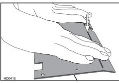
Using both screws previously removed, install the metal shutoff plate on top of the hood.
