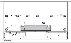
Fold down the foldable flange of the adapter/damper. This flange must be at 90° from the remaining flanges. See picture beside.
