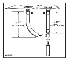
Cut 2 sections of plastic tubing, about 12" (305 mm) long and attach them to each drain fitting. Join these 2 short sections to the "T" junction and main tube as shown.
