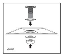
Attach both plastic drain fittings to the unit using the gaskets, washers and nuts as shown.
