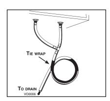
Make a water trap loop in the tube to prevent the unit from drawing unpleasant odors from the drain source. Make sure this loop is situated BELOW the "T" as shown. This will prevent water from being drawn back up into the unit in case of negative pressure. Run the tubing to the floor drain or to an alternative drain pipe or pail. Be sure there is a slight slope for the run-off.
