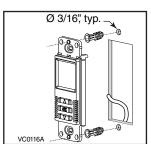
4. Strip the end of the cable to access the 4 wires. Strip the end of each wire. Using a small flat blade screwdriver, connect each wire to its corresponding terminal on the back of the wall control: YELLOW wire to "Y," RED wire to "R," GREEN wire to "G" and BLACK wire to "B."
