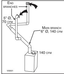
NOTE: A 4" Ø duct would have been too small because the maximum acceptable value for a 4"Ø duct is 60 cfm.
